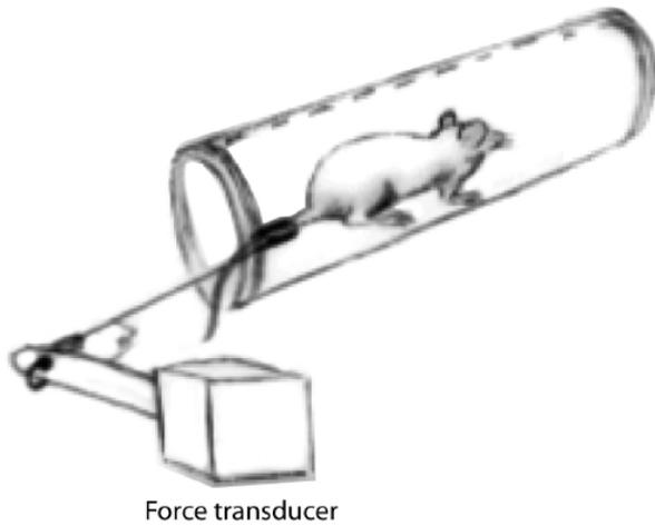
**Figure 1.** Diagram showing mouse position inside the tube with tail attached to a force transducer. Note that the tube walls are not normally transparent and are shown here as transparent only for purposes of illustration (drawing by Evelyn Carlson).
